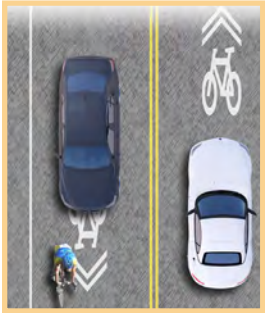
Shared Lane Marking
